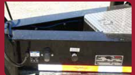
Conveniently located, easy to use controls for raising and lowering trailer and ramps.
