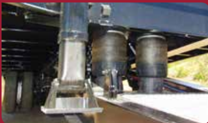
Pneumatically operated tilting deck and ramp design.
